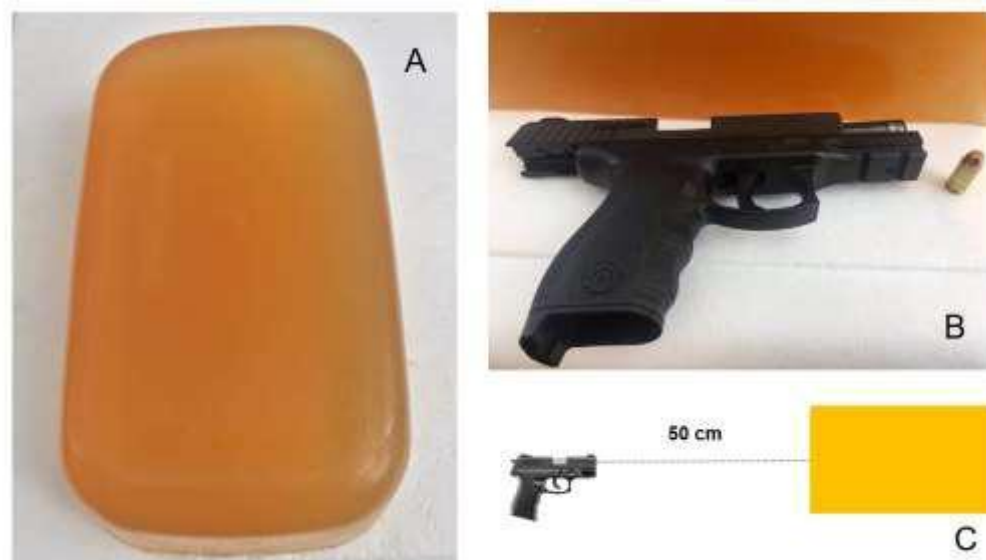
Figure 1. Ballistic gelatin block (10% gelatin) for the experimental test (A, B and C). (A) shows the gelatin block. (B) shows one of the guns used in the test (.40 S&W caliber). (C) shows the distance between the gun and the block.
