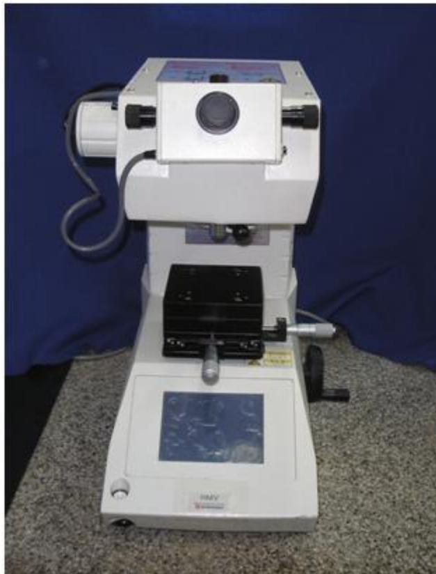
**Figura 6** - Microdurômetro (Shimadzu Micro Hardness Testers HMV-2 Series).
