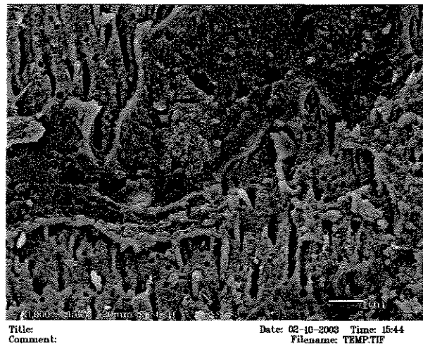
Figure 4. Representative micrograph (1000x) of interphase fracture from the one year storage groups. Tags in parallel directions are exposed, demonstrating a potential weakness of the hybrid layer after one year of storage.
