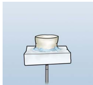
Fig. 3 Crown-segments glued to Plexiglass slabs.
