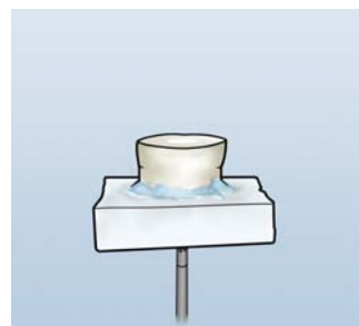
Fig. 3 Crown-segments glued to Plexiglass slabs.
