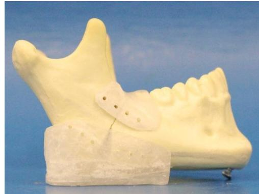
Figure 5 – Acrylic jigs used to reduce the fracture, guide and standardize the fixation
