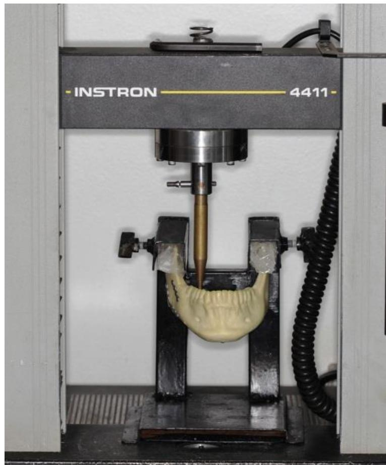
Figure 6 – A custom-made biomechanical testing model with a polyurethane mandible in the Instron 4411
