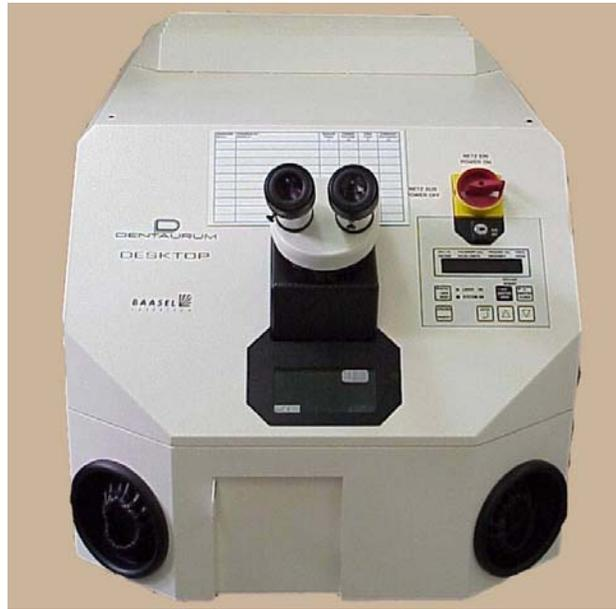
**Figura 8.** Máquina de solda a laser Desktop.
