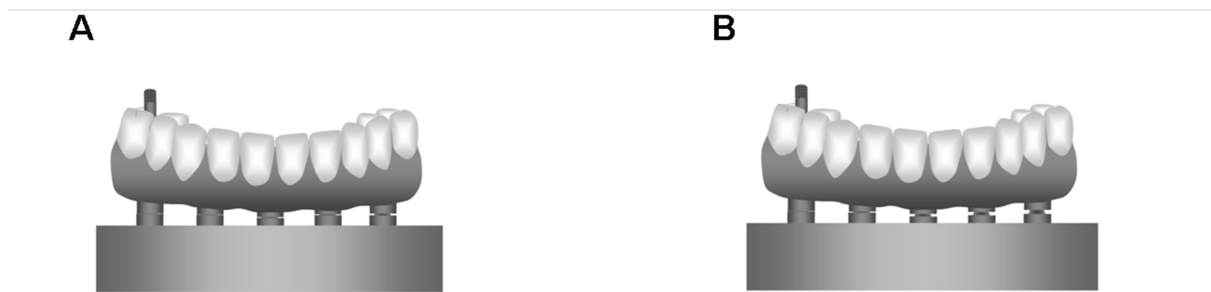
Figure 4. Schematic illustrations of the two fit conditions submitted to the one-screw test: (A) passive fit; (B) vertical misfit.
