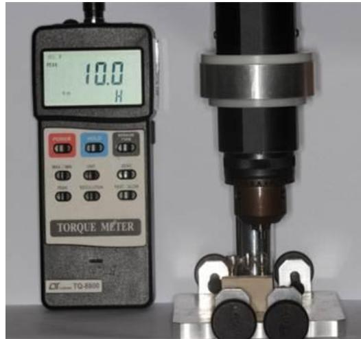
**Figure 2** – Digital torque meter and device to positioning.
