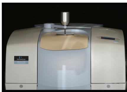
Figura 40: Aparelho FT-IR (Spectrum 100, Perkin Elmer).
