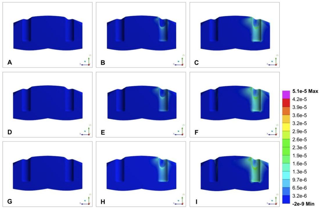
**Figure 4.** Maximum principal elastic strain (mm/mm) distribution in the peri-implant bone tissue for the bar cross-section geometries simulating horizontal misfits: (A) 10  $\mu\text{m}$ , (B) 50  $\mu\text{m}$ , and (C) 100  $\mu\text{m}$  using circular bar; (D) 10  $\mu\text{m}$ , (E) 50  $\mu\text{m}$ , and (F) 100  $\mu\text{m}$  using ovoid bar; and (G) 10  $\mu\text{m}$ , (H) 50  $\mu\text{m}$ , and (I) 100  $\mu\text{m}$  using Hader bar.
