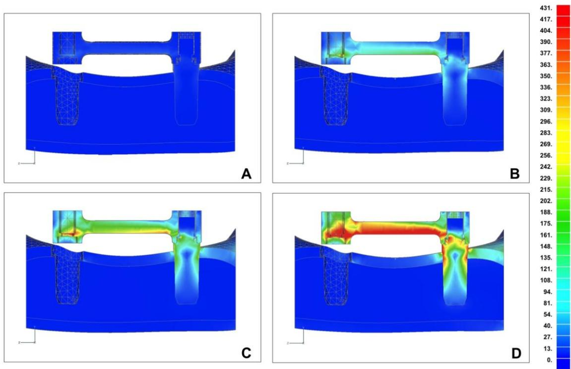
**Figure 2** Von Mises stress (MPa) distribution in the models with different horizontal misfits for the gold bar framework: (A) 10  $\mu\text{m}$ ; (B) 50  $\mu\text{m}$ ; (C) 100  $\mu\text{m}$ ; and (D) 200  $\mu\text{m}$ .
