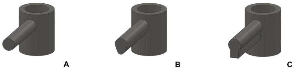
**Figure 1.** Design of the different cross-section geometry of the bar: (A) circular; (B) ovoid; and (C) Hader.
