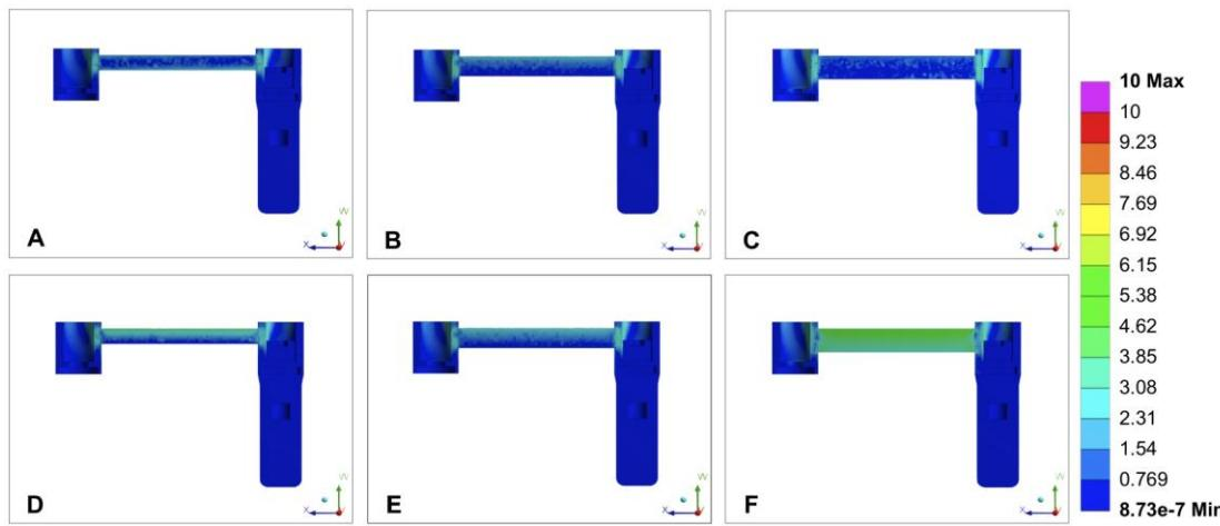
**Figure 5.** Von Mises stress (MPa) distribution in the mechanical part for bar cross-section geometries simulating different levels of bone loss and 50  $\mu\text{m}$  misfit: (A) circular bar, (B) ovoid bar, and (C) Hader bar without bone loss; (D) circular bar, (E) ovoid bar, and (F) Hader bar simulating 1.4-mm bone loss.
