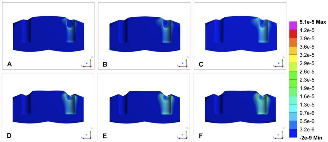
**Figure 6.** Maximum principal elastic strain (mm/mm) distribution in the peri-implant bone tissue for the bar cross-section geometries simulating different levels of bone loss and 50  $\mu\text{m}$  misfit: (A) circular bar, (B) ovoid bar, and (C) Hader bar without bone loss; (D) circular bar, (E) ovoid bar, and (F) Hader bar simulating 1.4-mm bone loss.
