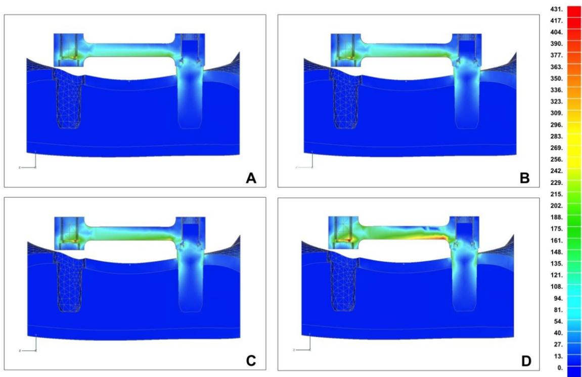
**Figure 3** Von Mises stress (MPa) distribution in the models with different bar framework materials for 50  $\mu\text{m}$  of misfit: (A) gold alloy; (B) silver–palladium alloy; (C) commercially pure titanium; and (D) cobalt–chromium alloy.
