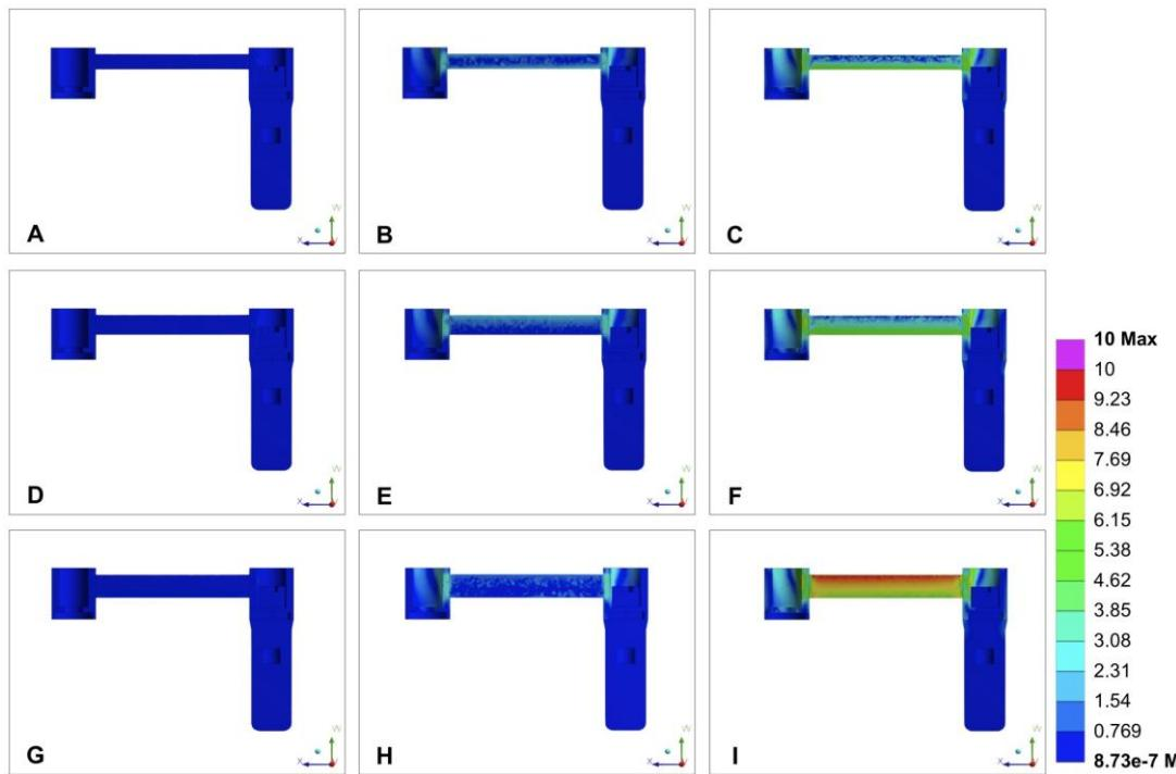
**Figure 3.** Von Mises stress (MPa) distribution in the mechanical part for the bar cross-section geometries simulating horizontal misfits: (A) 10  $\mu\text{m}$ , (B) 50  $\mu\text{m}$ , and (C) 100  $\mu\text{m}$  using circular bar; (D) 10  $\mu\text{m}$ , (E) 50  $\mu\text{m}$ , and (F) 100  $\mu\text{m}$  using ovoid bar; and (G) 10  $\mu\text{m}$ , (H) 50  $\mu\text{m}$ , and (I) 100  $\mu\text{m}$  using Hader bar.
