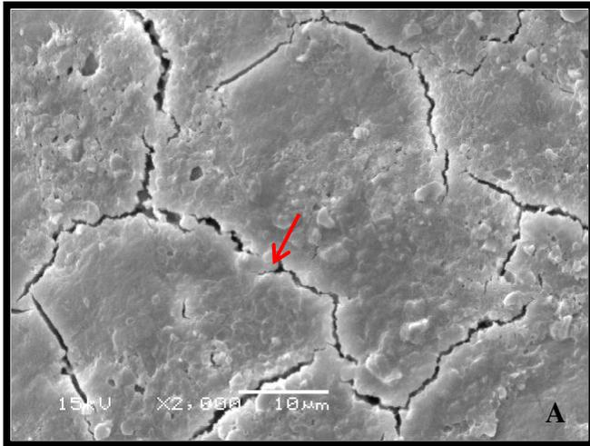
**Fig. 7.a. Laser 20.0 J/cm<sup>2</sup> + APF Group.** SEM micrograph after irradiation with 20.0 J/cm<sup>2</sup> on enamel and application of fluoride. Cracks, melting, fusion and calcium fluoride-like deposits are observed.
