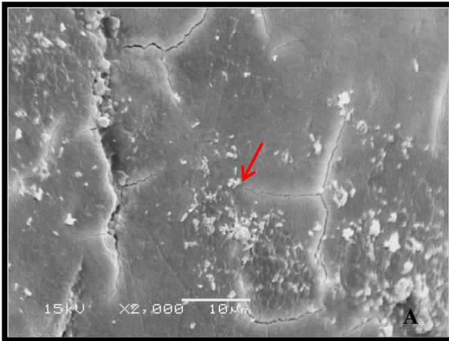
**Fig. 4.a. Laser 11.3 J/cm<sup>2</sup> + APF Group.** SEM micrograph after irradiation with 11.3 J/cm<sup>2</sup> on enamel and application of fluoride. Calcium fluoride-like deposits and cracks are observed.
