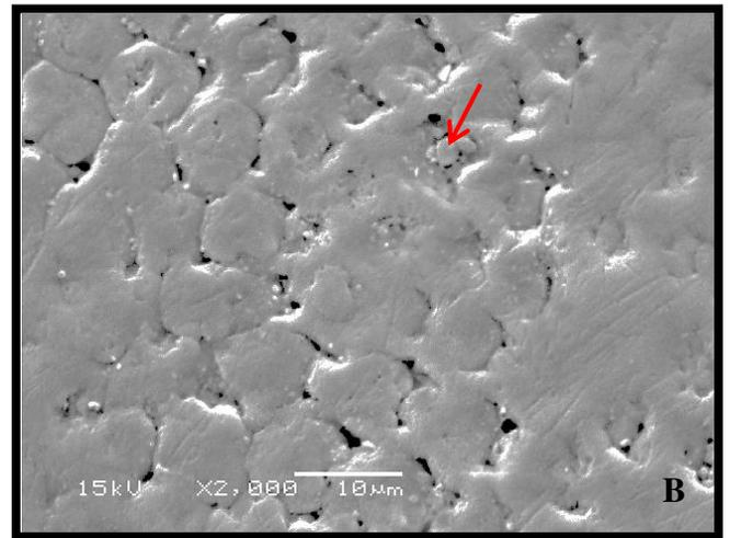
**Fig. 7.b. Laser 20.0 J/cm<sup>2</sup> + APF Group.** SEM micrograph after irradiation with 20.0 J/cm<sup>2</sup> on enamel, fluoride application and subsequent KOH treatment. No deposits are seen. Melting and fusion on surface are evident.
