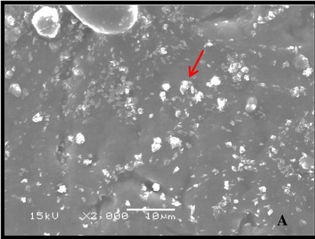
**Fig. 3.a. APF+Laser 11.3 J/cm<sup>2</sup> Group.** SEM micrograph after application of fluoride on enamel and irradiation with 11.3 J/cm<sup>2</sup>. Note the calcium fluoride-like deposits.
