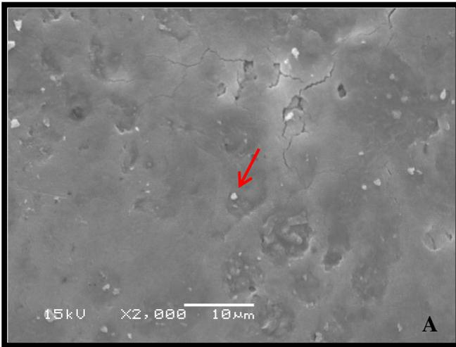
**Fig. 5.a. Laser 11.3 J/cm<sup>2</sup> + APF Group.** SEM micrograph after fluoride application during the irradiation with 11.3 J/cm<sup>2</sup>. Note the calcium fluoride-like deposits and surface alterations (melting and fusion).
