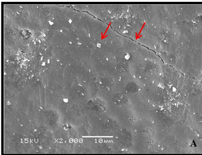
**Fig. 8.a. Laser 20.0 J/cm<sup>2</sup> + APF Group.** SEM micrograph after fluoride application during the irradiation with 20.0 J/cm<sup>2</sup>. Cracks, melting, fusion and calcium fluoride-like deposits are observed.
