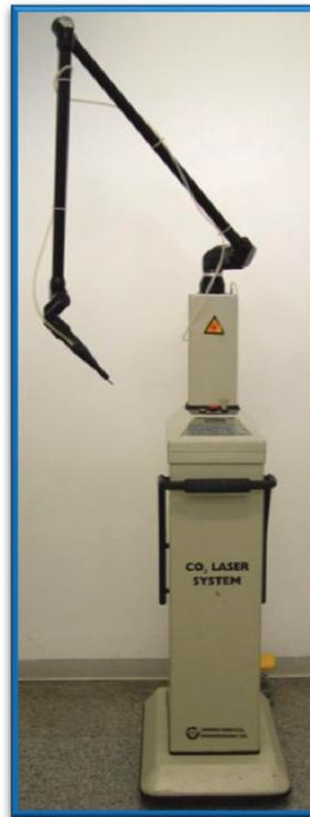
Figura1: Laser de CO<sub>2</sub> Union Medical Engineering Co. Model UM-L30, Yangju-si, Gyeonggi-Do, Korea)
