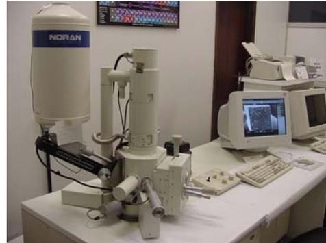
Figura 26 – MEV JSM – 5600 – JEOL, USA
