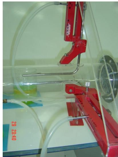
Figura 3.9 – Tubo de pitot na horizontal e vertical
