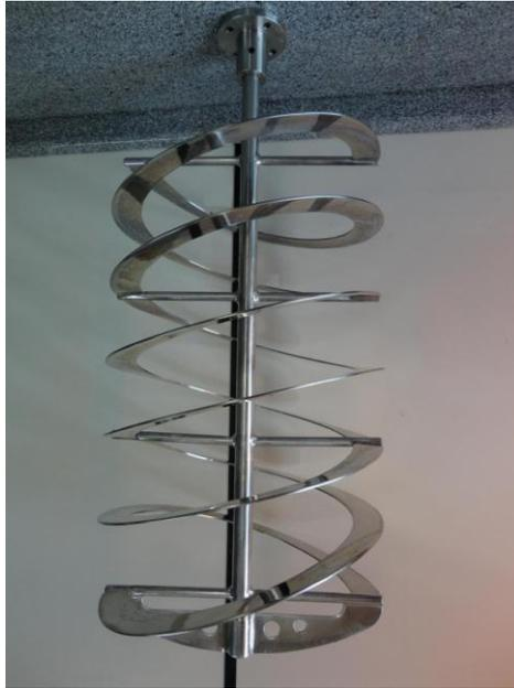
**Figura 2.10** Impelidor Helicoidal (L-CFD).
