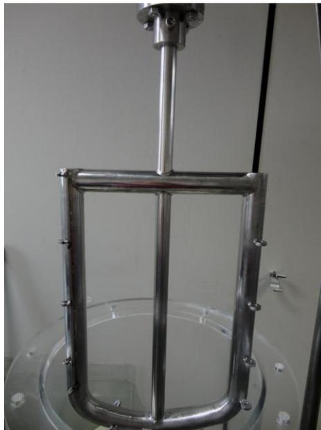
**Figura 2.9** Impelidor Âncora tubular (L-CFD).
