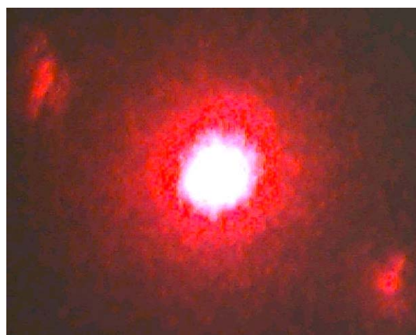
Fig. 5. Diffracted pattern of a laser beam in the same conditions above for dense membranes observed after solvent evaporation (drying step) and after coagulation, washing and drying at room temperature steps.
