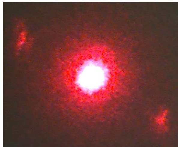
Fig. 4. Diffracted pattern of a laser beam as observed at a perpendicular screen placed 50 cm behind the film. The large central spot is the transmitted beam whereas both symmetric smaller lateral spots are the diffracted beams produced by the periodic structure in the film at the point of incidence of the laser beam for dense membranes observed after drying step.
