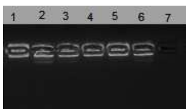
FIG 3: Agarose gel electrophoresis (1.5%) of pseudo-ternary HA/ cationic liposome/DNA complex at different molar HA amounts Lanes: 1)CL-DNA 2) HA/CL-DNA 0.25%;3) HA/CL-DNA 0.5%;4) HA/CL-DNA 1%;5) HA/CL-DNA 3%;6) HA/CL-DNA 5%;7) HA/CL-DNA 30%. The molar charge ratio between the ECL and DNA used was R_{+/-} = 3
