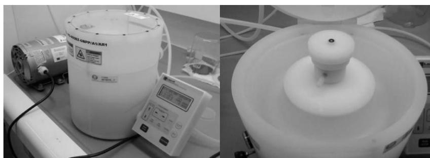
Figura 1. Spin coater da marca Laurell (modelo WS-400BZ-6NPP/A1/AR1)
