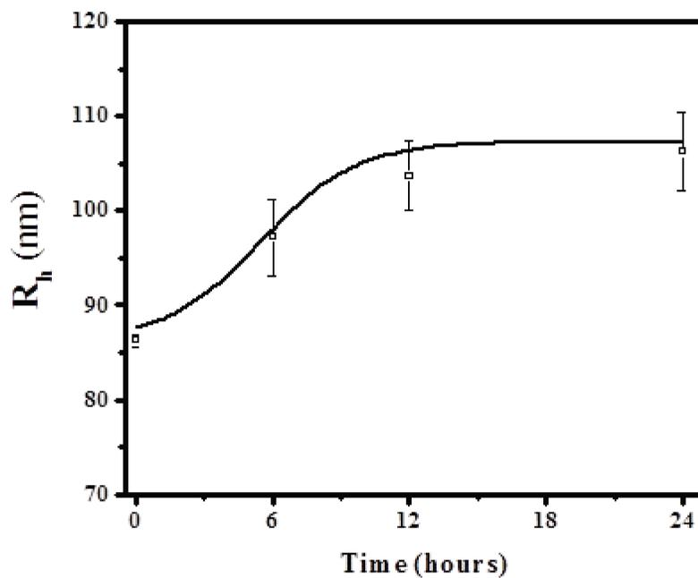
**Figure 7.**  $R_h$  vs. time of the SLN in presence of  $45 \text{ mg}\cdot\text{mL}^{-1}$  HSA dissolved in PBS. Microscopy images analyzed by TEM and SEM of empty SLN are presented in Figure 8. SLN showed spherical morphology.
