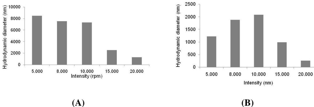
**Figure 1.** Influence of Ultra-Turrax® intensity on the particle size of the pre-emulsion to produce (A) SLN and (B) NLC.
