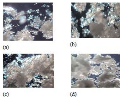
**Figure 3.** Micrographs obtained by PLM of stearic acid (a) and of stearic acid-capric/caprylic triglycerides (b) before tempering; and of stearic acid (c) and stearic acid-capric/caprylic triglycerides (d) after tempering.
