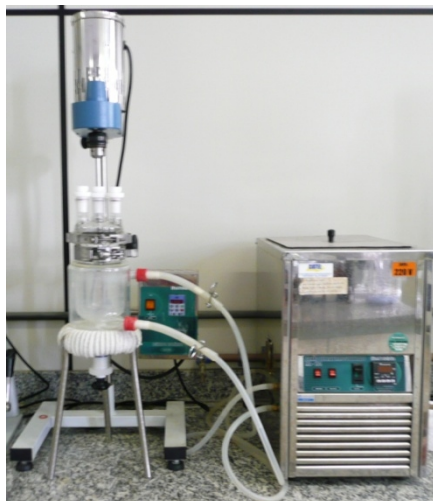
Figure 1. Experimental set-up for transesterification of castor oil
