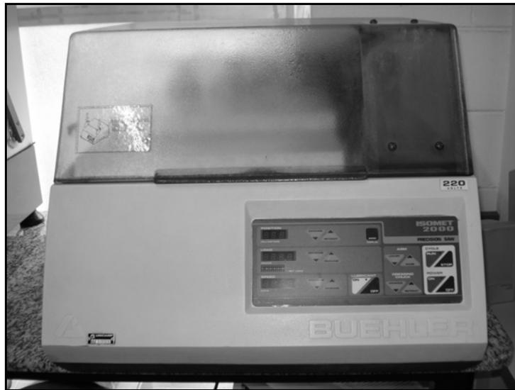
**Figura 3.3** – Cortadeira ISOMET 2000<sup>®</sup> Precision Saw.
