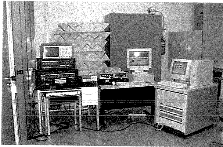
Figure 5.3: Devices used in the experimental set up – 3 power amplifiers, 2 analog filters, 1 function generator, 1 oscilloscope, 1 signal conditioning unit, 1 DSP control board and 1 spectral analyzer.
