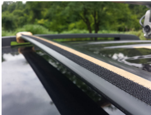
Figure 4.21: Turbulence Mesh Boundary Layer Tripping detail.
