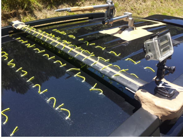
(a) Tufts of yarn and camera installation.
