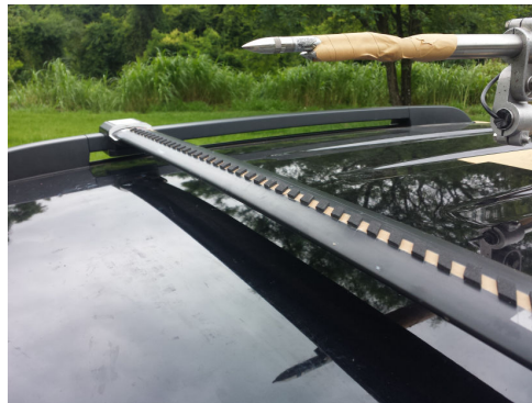
Figure 4.27: 3D Boundary Layer Tripping on Elliptical cylinder.
