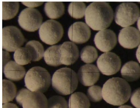
**SEM.** The surface morphology of BCP microspheres after sintering is shown in Fig. 4. The surface roughness of the spheres and the interconnected pores of the sintered particles can be clearly seen.
