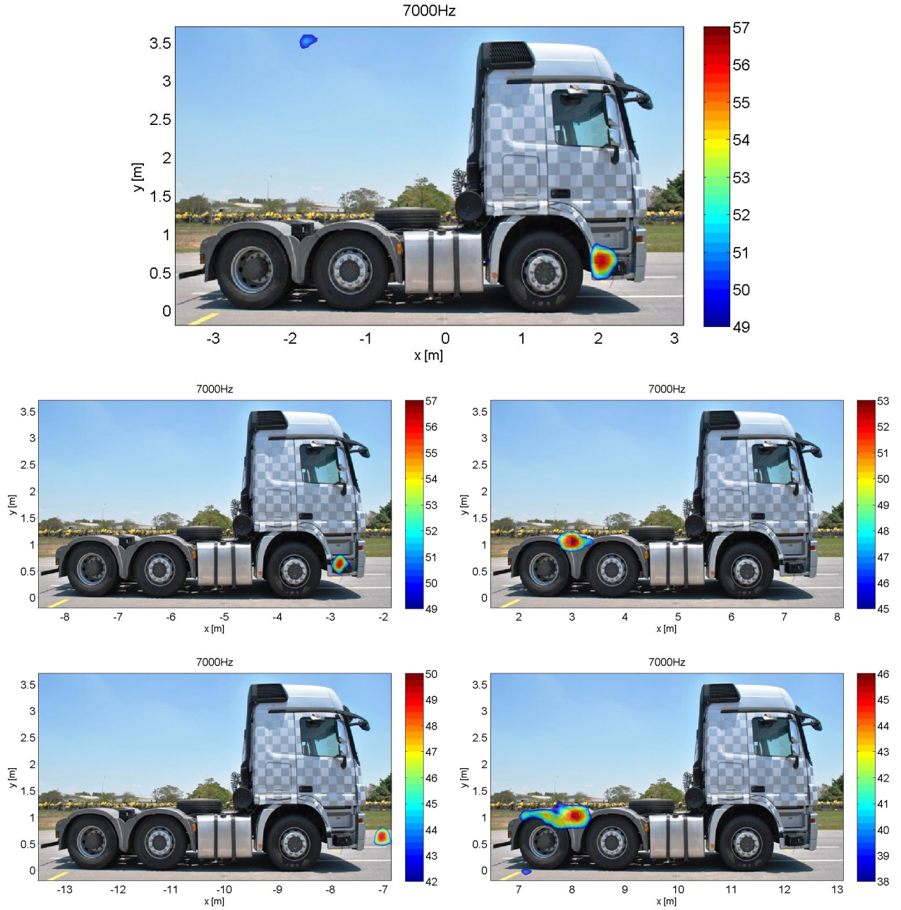
Figure 10.20: Identifications on 7kHz 3 rd oct. of front and rear loudspeakers with incoherent white noise using IRLS scheme and truck at constant speed of 50km/h for various track positions. Mappings are 3 rd oct. SPL (A-Weighted) at pass-by noise microphone position.
