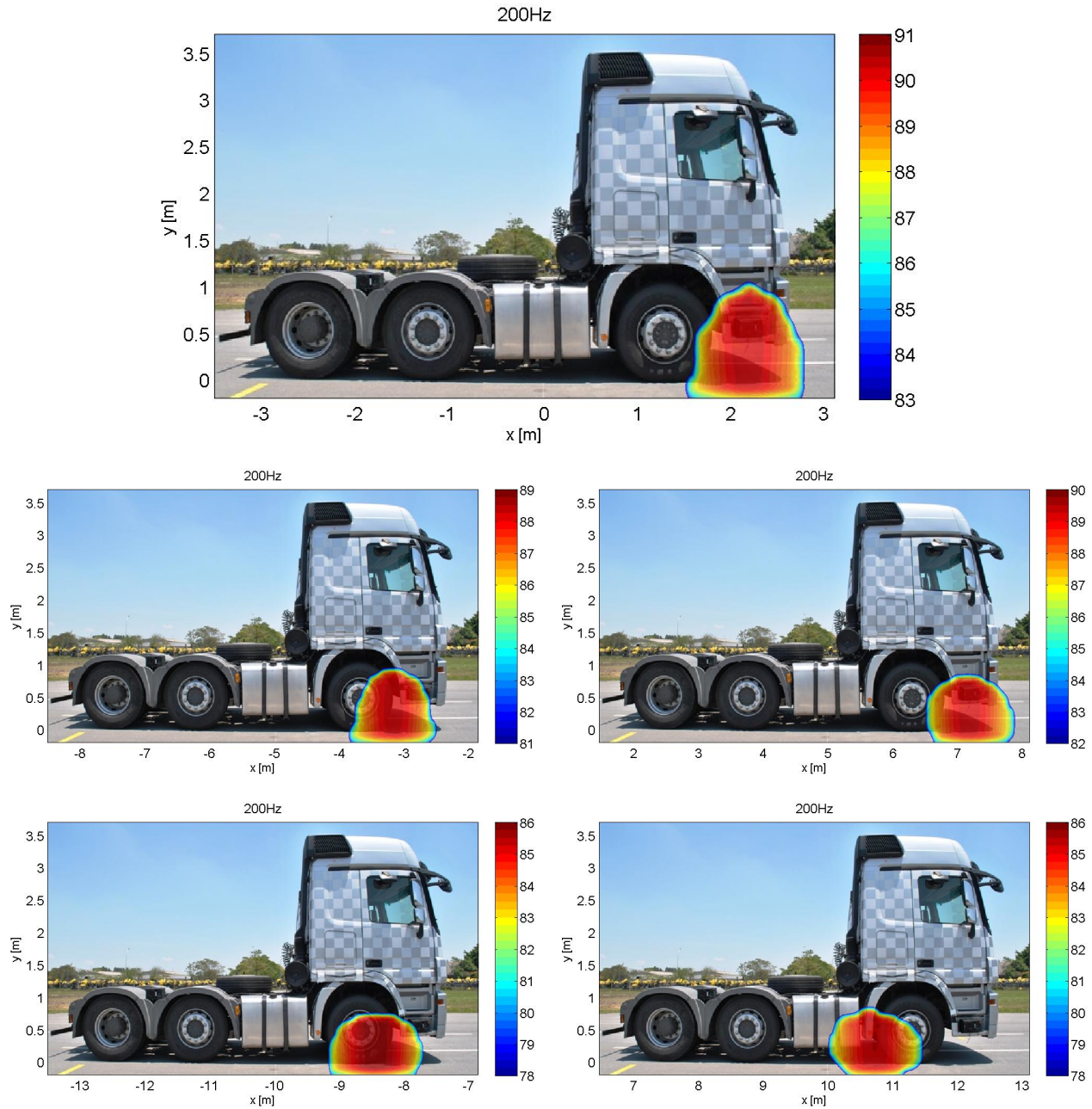
Figure 10.11: Identifications of front loudspeaker with tonal 200Hz using low frequency focus compensation and truck at constant speed of 50km/h for various track positions. Mappings are 3 rd oct. SPL (A-Weighted) at pass-by noise microphone position.
