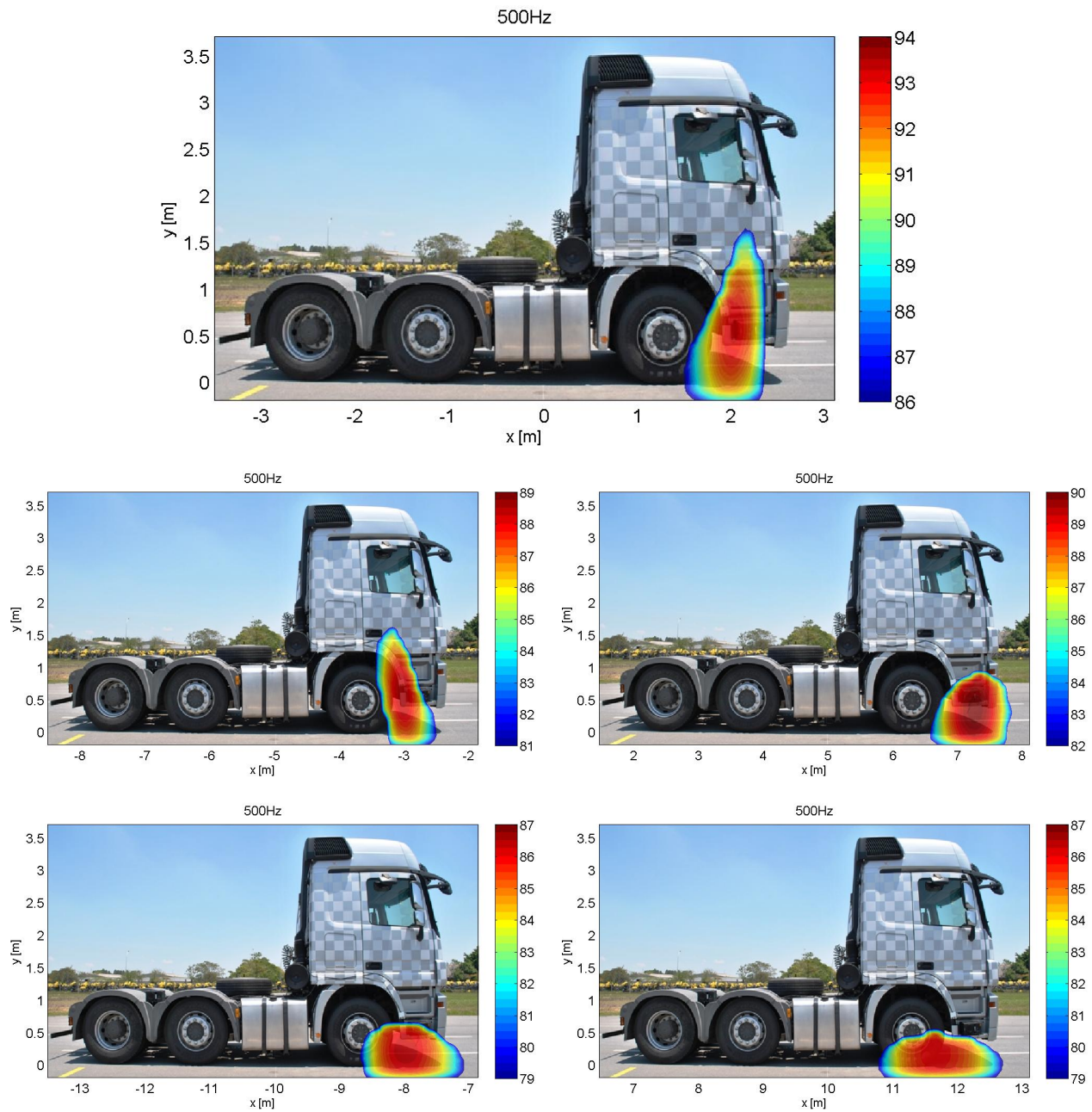
Figure 10.8: Identifications of front loudspeaker with tonal 500Hz using image source in transfer matrix and truck at constant speed of 50km/h for various track positions. Mappings are 3 rd oct. SPL (A-Weighted) at pass-by noise microphone position.
