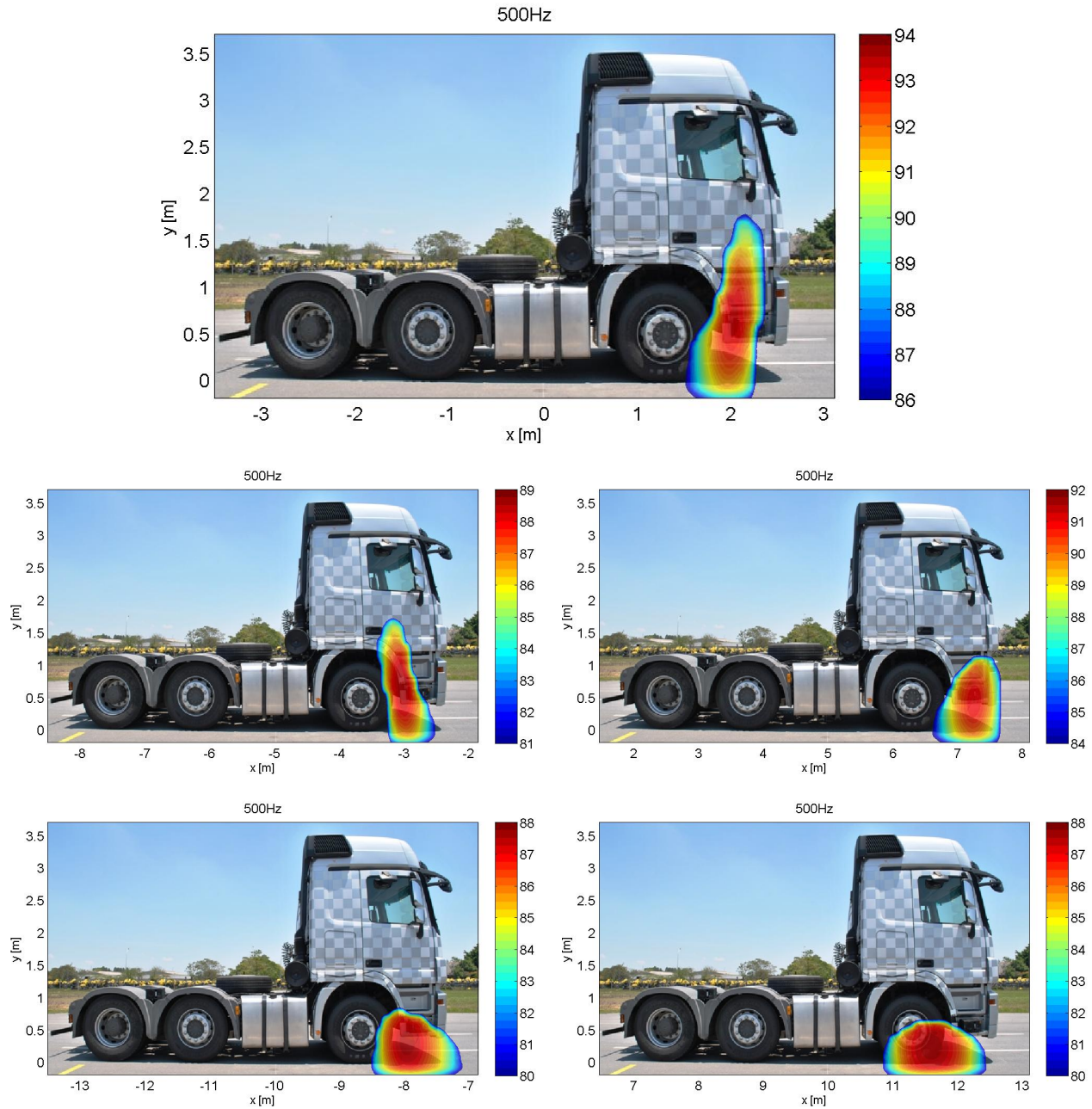
Figure 10.7: Identifications of front loudspeaker with tonal 500Hz and Truck at constant speed of 50km/h for various track positions. Mappings are 3 rd oct. SPL (A-Weighted) at pass-by noise microphone position.
