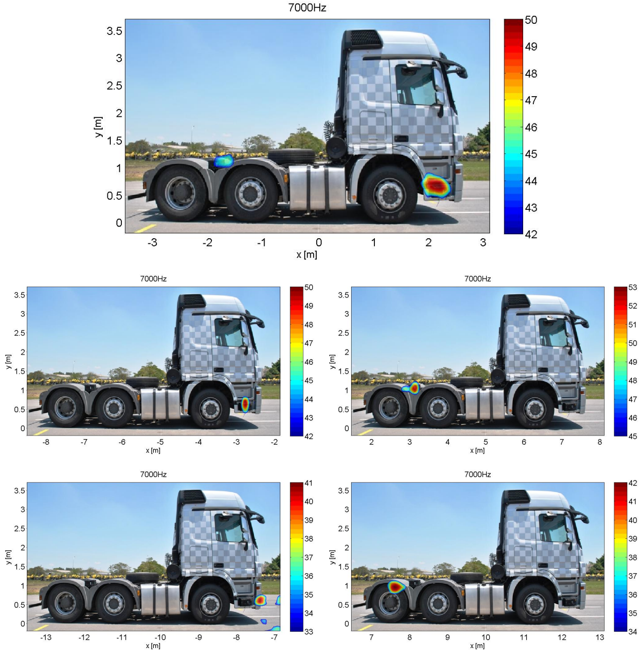
Figure 10.19: Identifications on 7kHz 3 rd oct. of front and rear loudspeakers with coherent white noise using IRLS scheme and truck at constant speed of 50km/h for various track positions. Mappings are 3 rd oct. SPL (A-Weighted) at pass-by noise microphone position.
