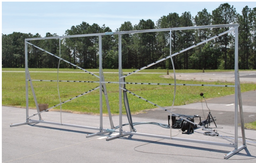
Figure 10.3: Array assembly with 61 microphones, including pass-by noise microphone position at array center.
