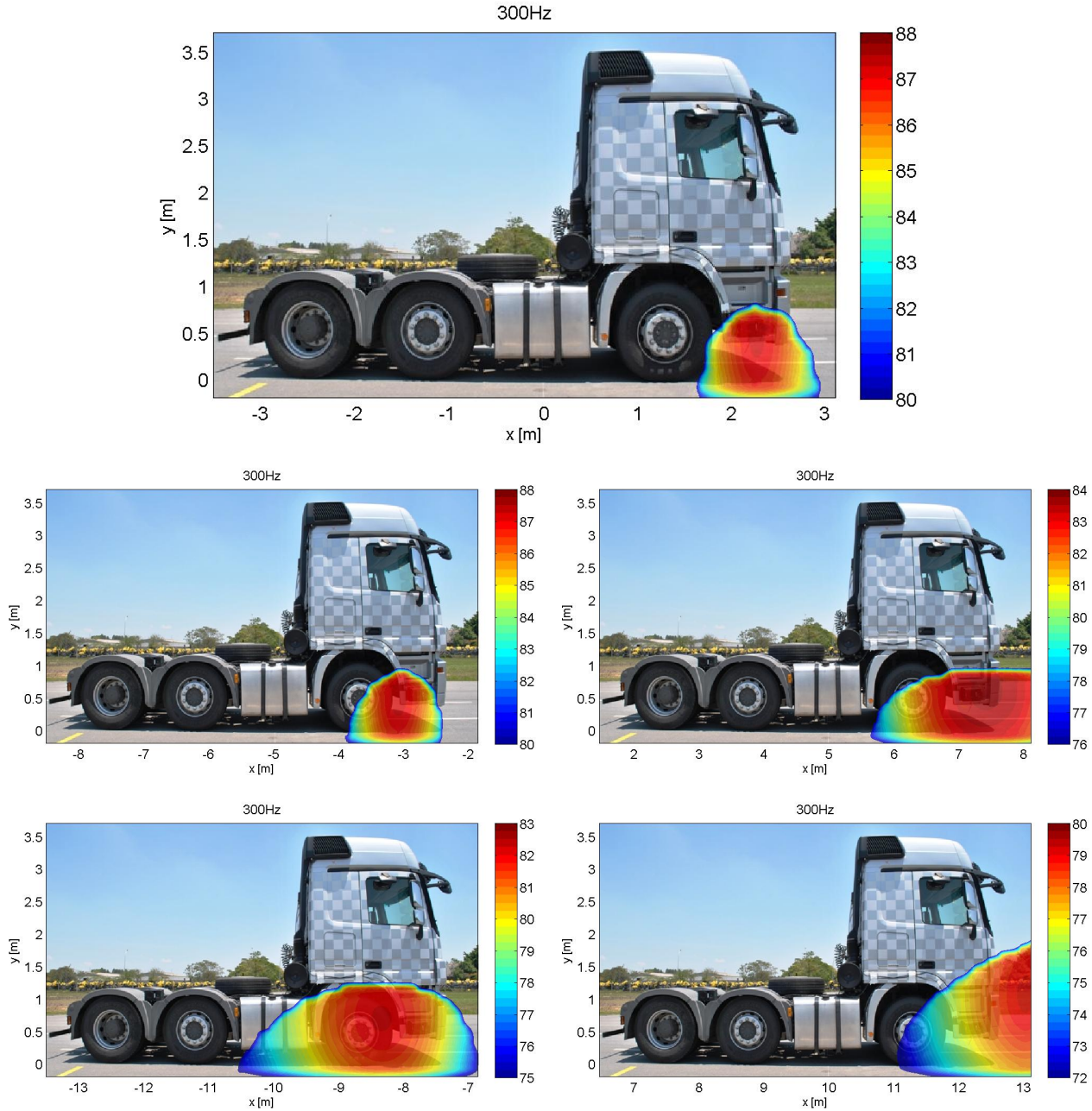
Figure 10.17: Identifications of front loudspeaker with tonal 300Hz using IRLS scheme and truck at constant speed of 50km/h for various track positions. Mappings are 3 rd oct. SPL (A-Weighted) at pass-by noise microphone position.
