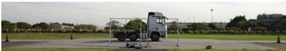
Figure 10.3: Array assembly with 61 microphones, including pass-by noise microphone position at array center.
