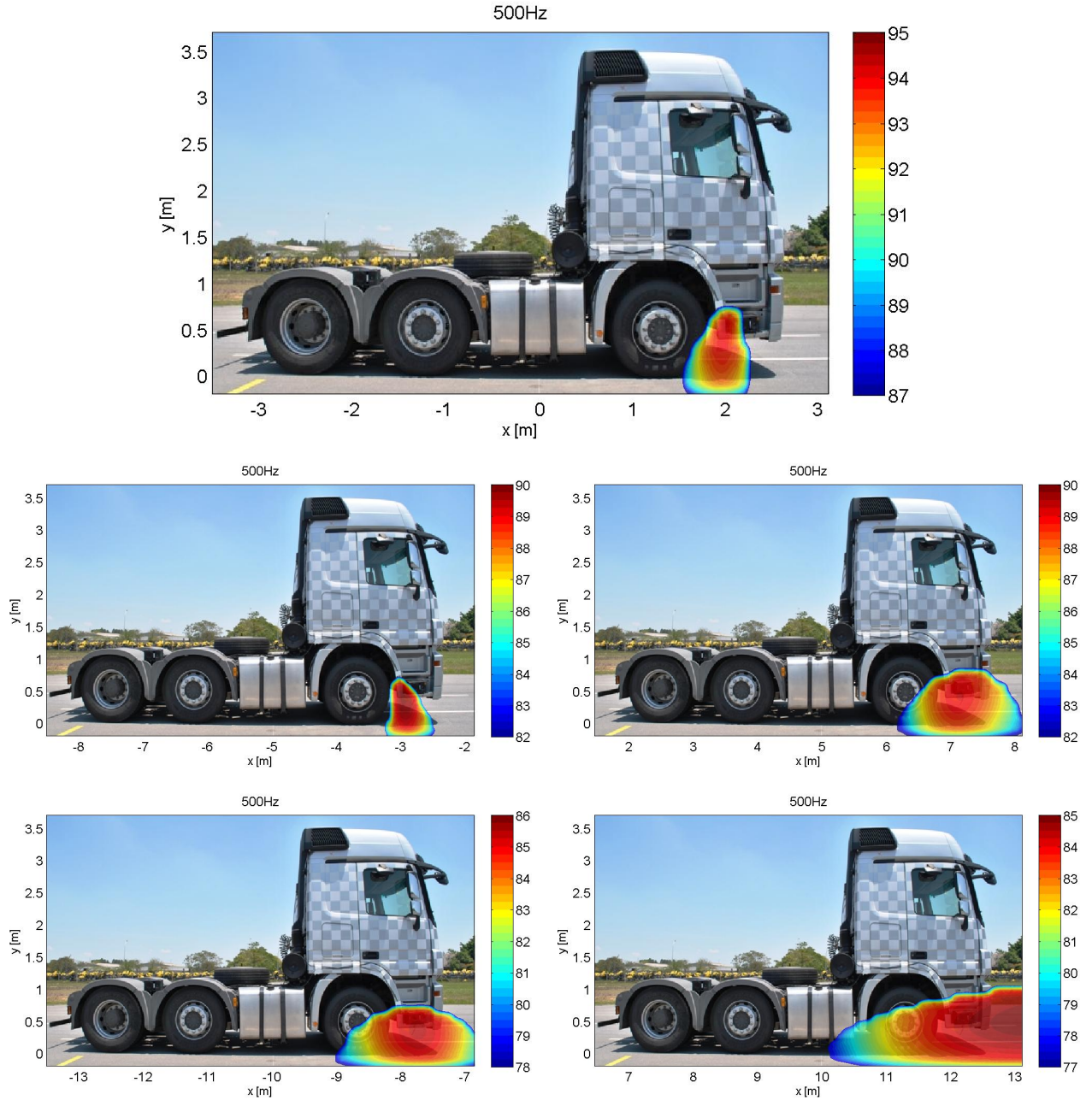
Figure 10.16: Identifications of front loudspeaker with tonal 500Hz using IRLS scheme and truck at constant speed of 50km/h for various track positions. Mappings are 3 rd oct. SPL (A-Weighted) at pass-by noise microphone position.
