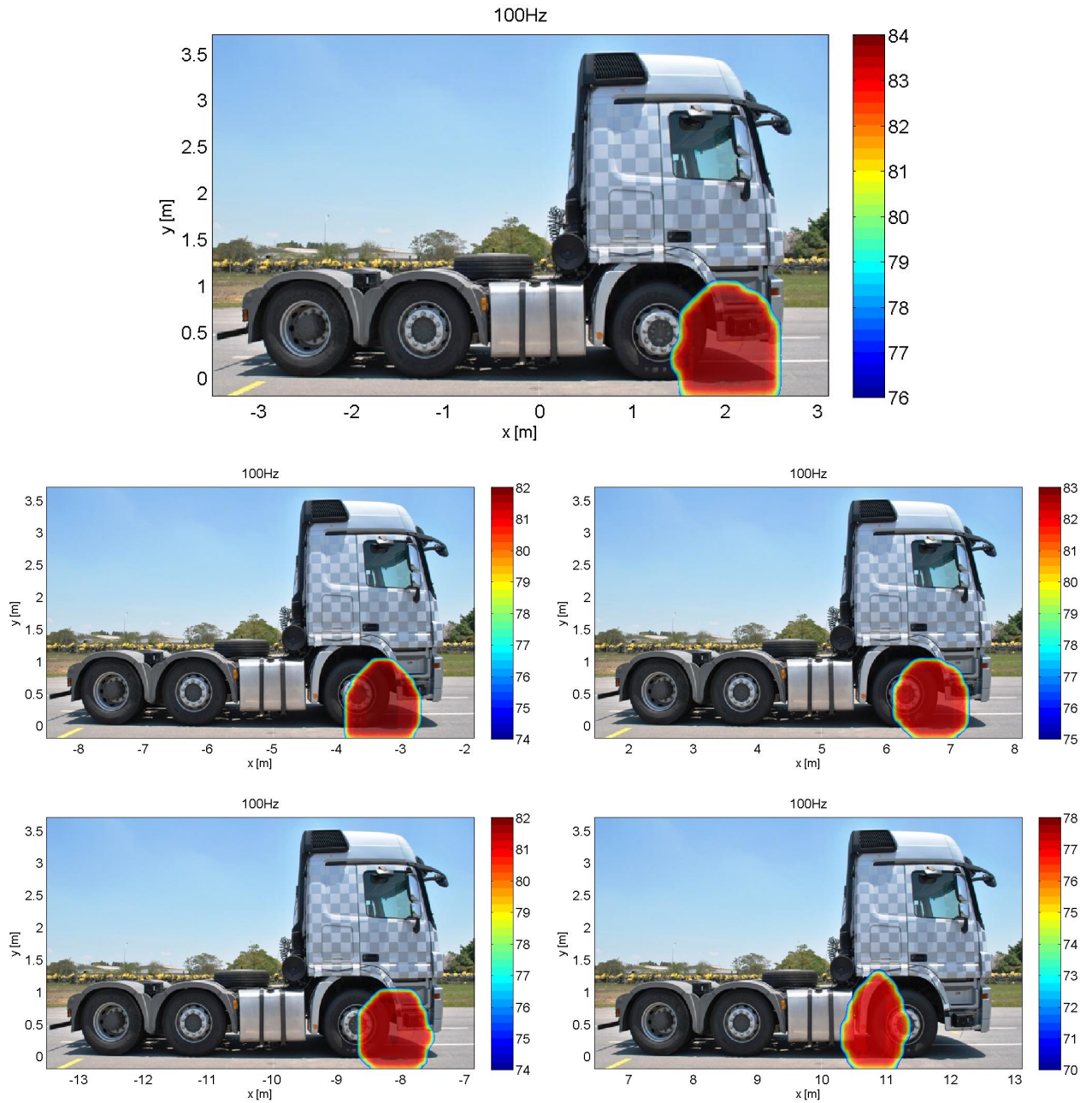
Figure 10.12: Identifications of front loudspeaker with tonal 100Hz using low frequency focus compensation and truck at constant speed of 50km/h for various track positions. Mappings are 3 rd oct. SPL (A-Weighted) at pass-by noise microphone position.
