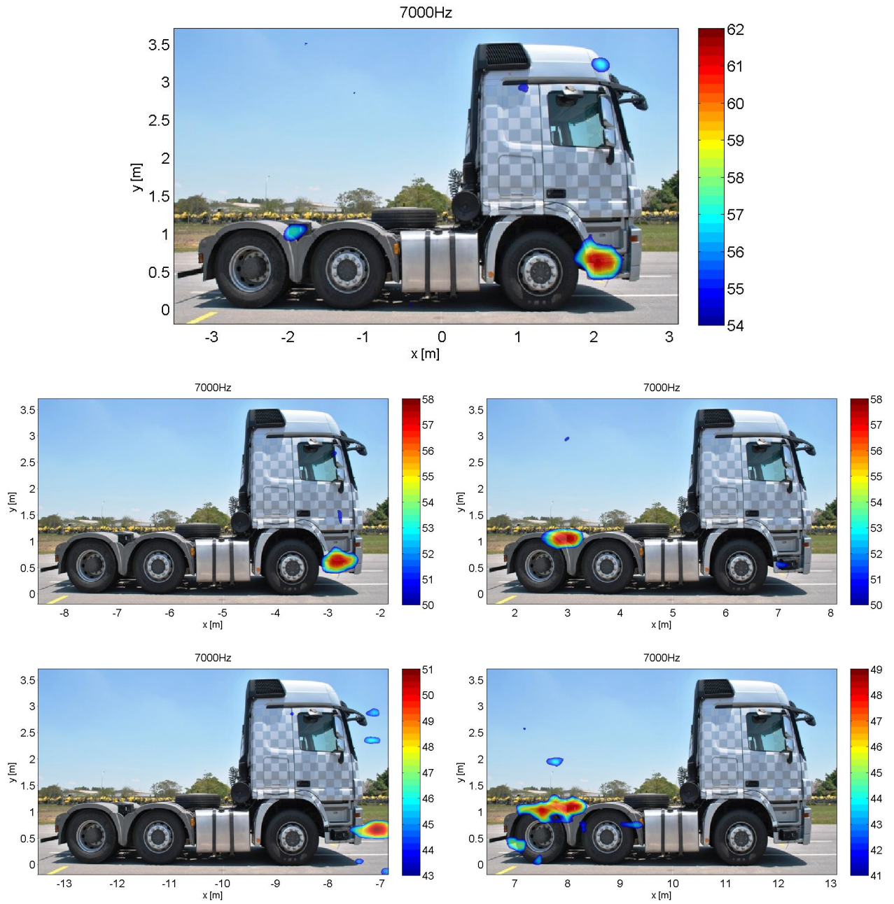
Figure 10.15: Identifications on 7kHz 3 rd oct. of front and rear loudspeakers with incoherent white noise and truck at constant speed of 50km/h for various track positions. Mappings are 3 rd oct. SPL (A-Weighted) at pass-by noise microphone position.
