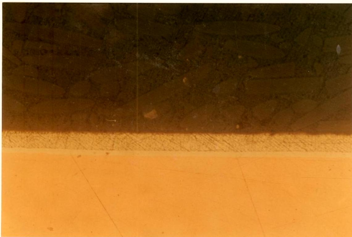
**Foto 02** - Depósito Zn-1%Fe ,  $I = 17 \text{ A/dm}^2$  ,  $t_{\text{dep}} = 5$  minutos ,
