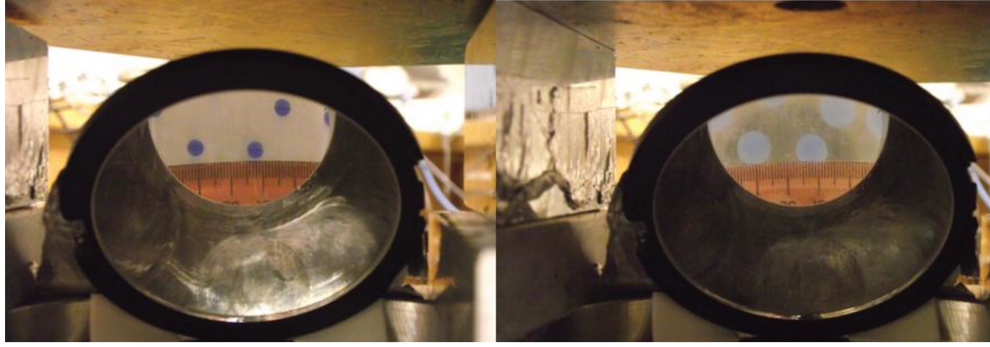
Figure 18: Diameter of inclusions under no pressure (left) and 13 MPa pressure (right).
