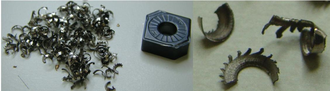
**Figura 4.2.4: Ferramenta CNMX 12 04 A2 – SM 1105  $v_c$ : 40m/min, f:0,10mm/volta,  $a_p$ :0,5mm**
