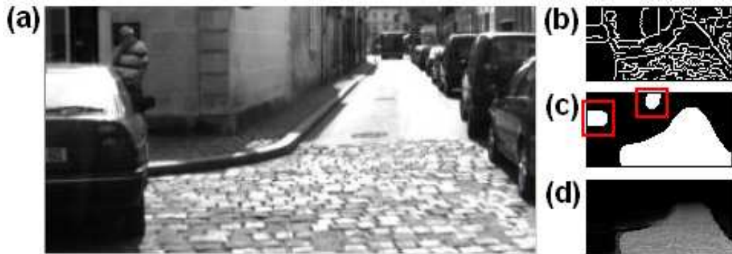
Figure 3.8 – (a) Original image after sky removal and its Otsu's result in (c); (b) Canny edge detection result; (d) A multimodal 2D drivability road image by considering the drag process:
