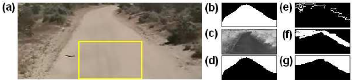
Figure 3.6 – (a) Original image and its Otsu's result in (b); (c) negated image and its Otsu's result in (d); (e) Canny edge detection result; (f) Hough transform result; (g) a single mass in the image (f).
