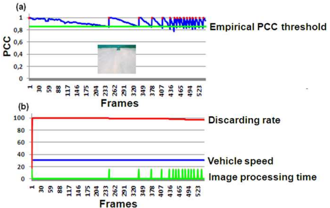
Figure 2.4 – DARPA Desert text-set 1 (DARPA, 2005): (a) Green line: empirical PCC threshold equal to 0.85; Above of the green line it presents the discarded images; Red points: reference frames; (b) Red line: discarding rate; Blue line: vehicle speed; Green line: hypothetical image processing time (15ms).
