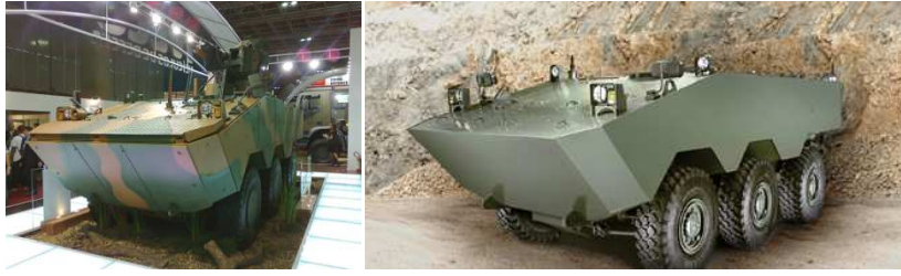
Figure 1.6 – The VBTP-MR: a 6x6 armored personnel carrier jointly developed by Fiat's IVECO and the Brazilian Army (VBTP-MR Project, 2011).
