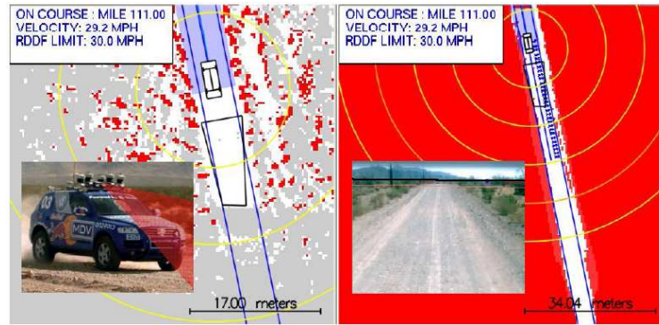
Figure 2.2 – Monocular vision: comparison of the laser-based (left) and the image-based (right) mapper. Circles are spaced around the vehicle at 10 meters distance. It includes the sky removal process.
