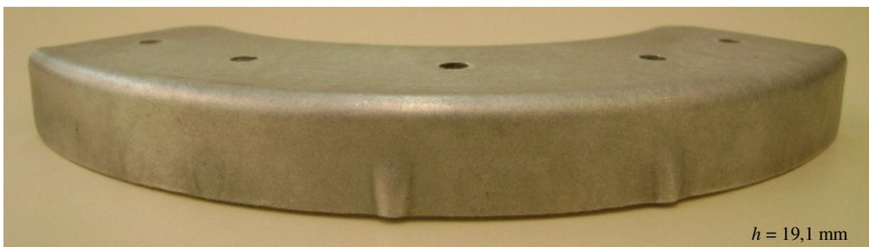
Figura 4.5 – Componente com rugas acima do limite ( $R_C=100 \text{ mm}$ ;  $e=1,0 \text{ mm}$ ).
