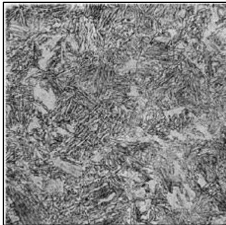
Figura 4.4 – Aço AISI S4 martensita e bainita 4% picral (500x) (ASM HANDBOOK, 2004)
