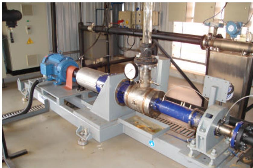
Figura V.2 – Skid de BCSs: motor, torquímetro e BCS.
