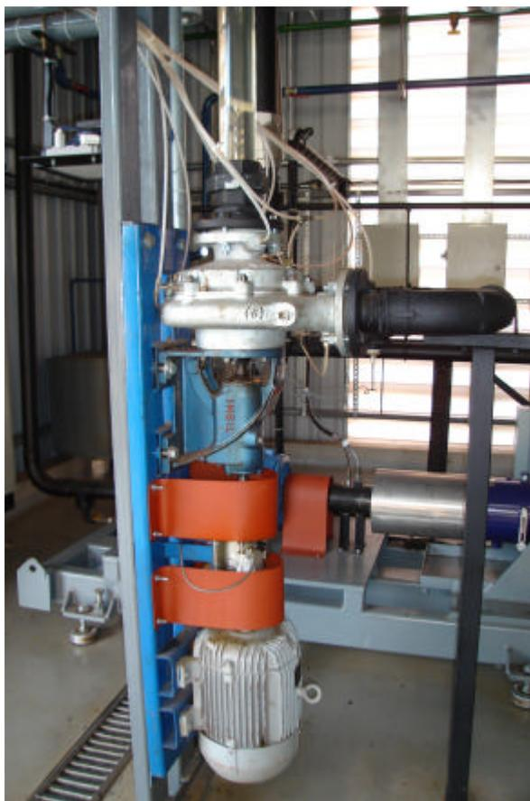
Figura V.5 - Skid vertical com a bomba Imbil ITA 65-330/2.
