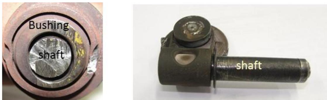
**Figure 1.2 - Wear between bushing and shaft.**
