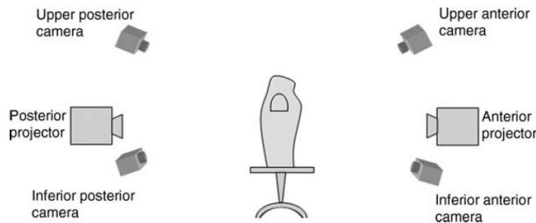
Figure 2. Experimental set-up used for images acquisition showing the arrangement of the cameras, projector and the subject/mannequin.
