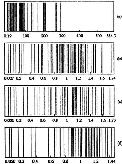
Figure 4: *Impact of pre-conditioning on eigenvalue spectrum for the IEEE-118 network.*
