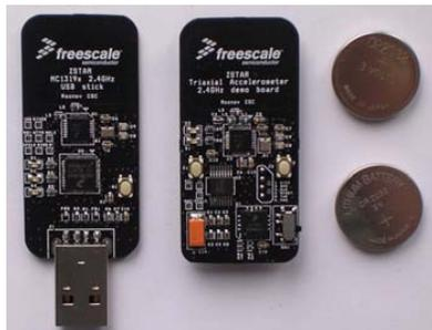
Fig. 12. Picture of ZSTAR DEMO board from Freescale.
