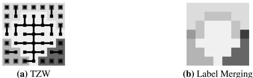
Fig. 3.5: **(a)**: TZW applied on image  $I_3$  of Figure 3.2 using 4-adjacency: 3 CBs (grey), TZ (white), a possible forest (black). **(b)**: Result of the Label Merging algorithm.
