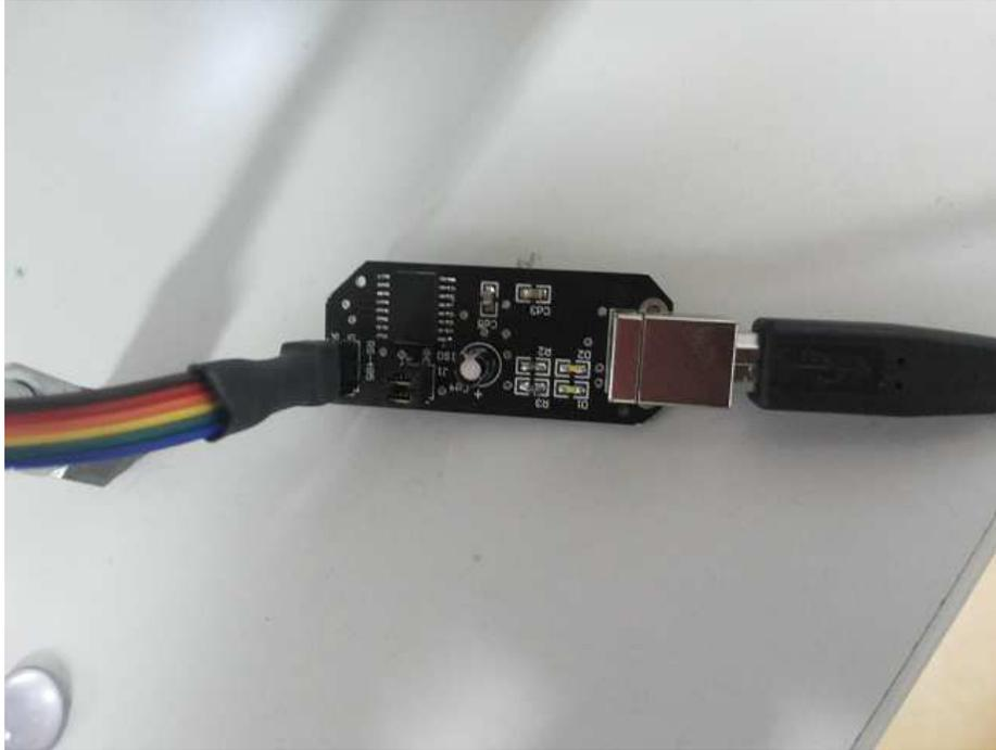
Figure 3.12: Picture of the interface and isolation board.
