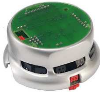
Fig. A.1: Mini-robô Khepera II (adaptado de www.k-team.com )
