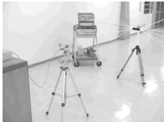
Fig. 12. 3m-Far-Field Measurement Setup
