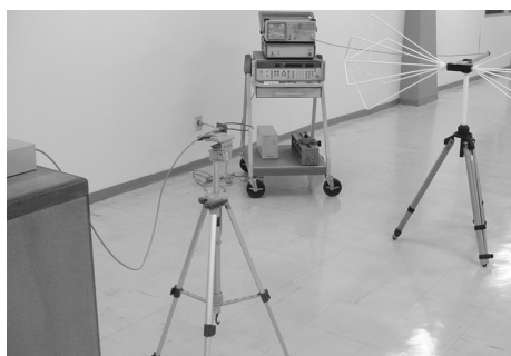
Fig. 11. 3m-Far-Field Measurement Setup
