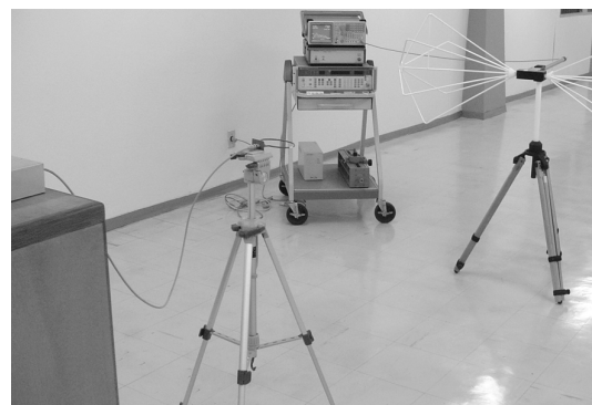
Fig. 9 Basic Antenna Setup and Electric Field Measurement
