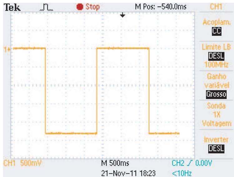
Fig. 4.10: Measured result in the output of the op-amp (clock signal of the ADG819 switches).
