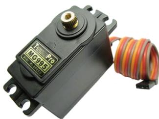
Figura 5.30: Servomotor TowerPro MG995.
