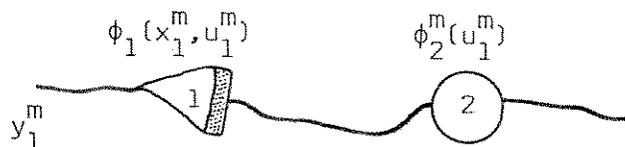
$$\begin{aligned} \phi^m(x^m, u^m) &= \phi_1(x_1^m, u_1^m) + \phi_2(u_1^m + y_2^m) = \\ &= \phi_1(x_1^m, u_1^m) + \phi_2^m(u_1^m) \end{aligned}$$
