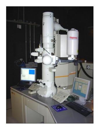
Figure 2.1 - The JEM 2100 transmission electron microscope manufactured by JEOL (Tokyo, Japan) installed at LNNano. Acceleration voltage: 200 kV. The electron source is a LaB<sub>6</sub> crystal. Source: LNNano website<sup>1</sup>.
