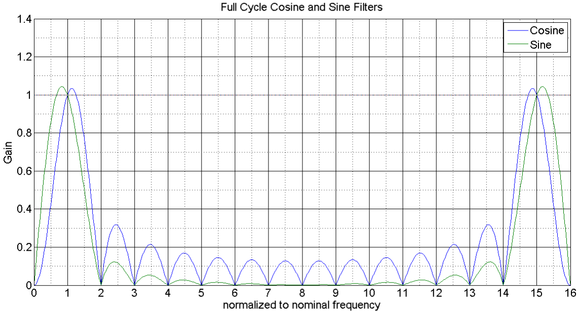
Figure C.2.6 – Digital filter response for one cycle window
