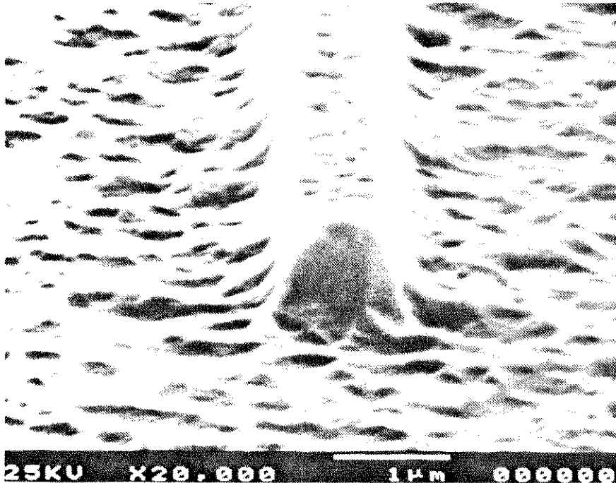
Figure 8 : Tungsten surface and wall profile for partial etching with a SF 6 - 50% O 2 plasma.
