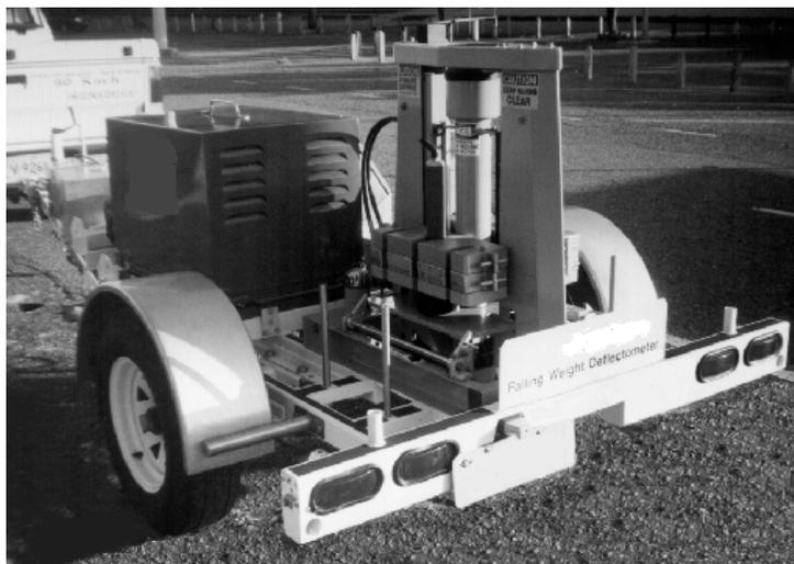
**Figura 2.3 - FWD - *Falling Weight Deflectometer***
