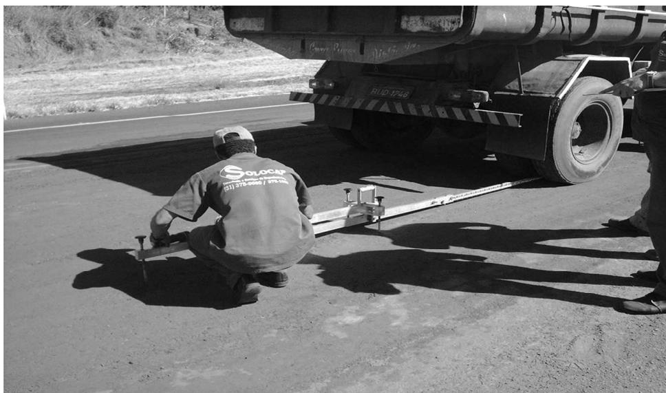
Figura 2.1 - Viga Benkelman
