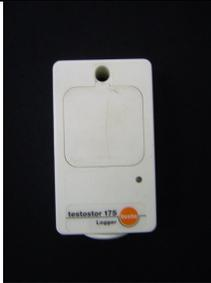
A photograph of a white, rectangular mini data logger. It has a small circular sensor at the top and a small display or indicator at the bottom. The text 'testostor 175' is visible on the front.                                                                    | Testostor 175-1 - Mini data logger<br>Modelo 0577 1751<br>Testo do Brasil –Equipamentos de Medição Ltda<br>1 canal: temperatura<br>Resolução de 0,1 ° C                              |
