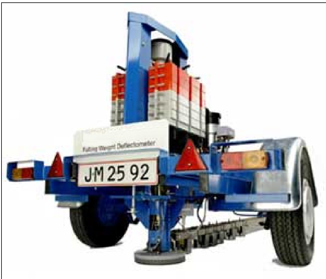
Figura 3.20 – Equipamento Dynatest FWD. Fonte: site http://www.dynatest.com/ .
