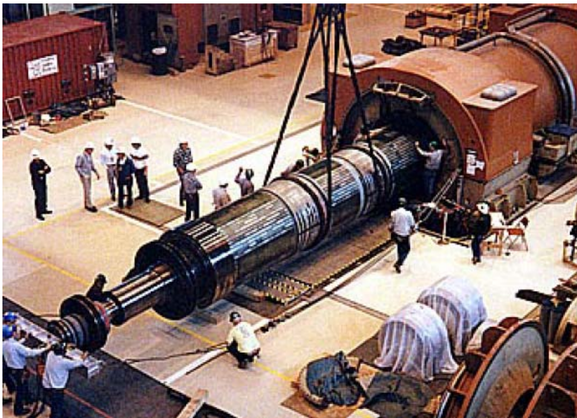
Figura 1.3.f: Montagem de rotor de turbogerador (adaptado de P. C. Sen, Principles of electric machines and power electronics)
